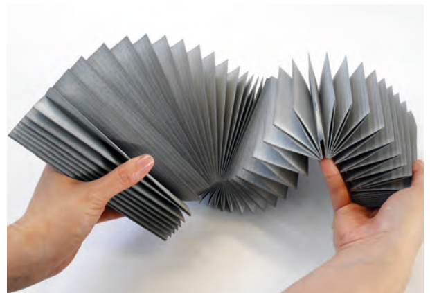
Figure 6: Accordion structure composed of a number of connected plates
