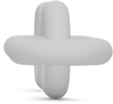
Figure 8: Chain links oriented at 0 and 90 degrees to the print bed
