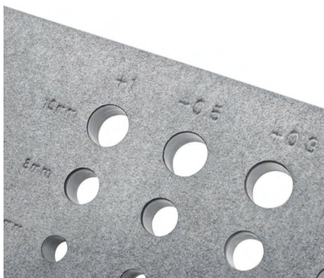
Figure 2: HP MJF pre-formed hole testing
