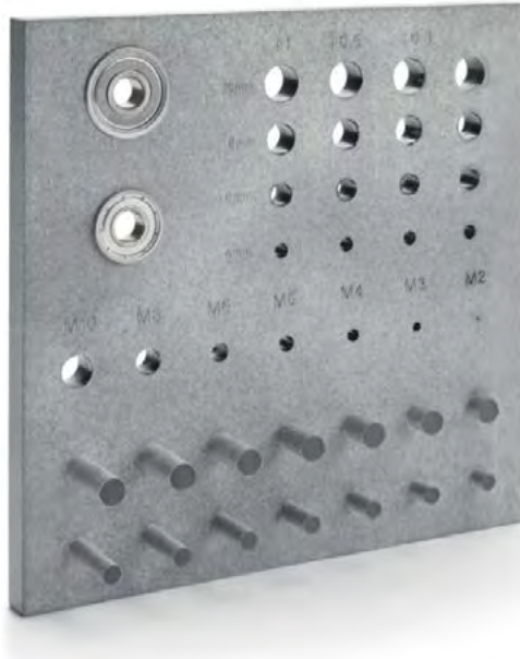
Figure 3: Bearings inserted into an HP MJF part
