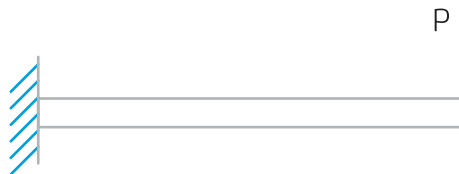
Figure 10. Cantilever beam with a point-applied end load
