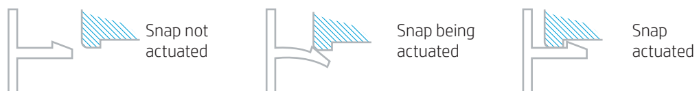
Figure 2. Cantilever snap-fit assembly operation
