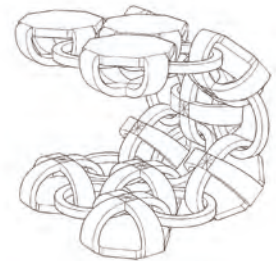
Figure 23: The folded elements shown here are bent 45, 90, and 135 degrees.
